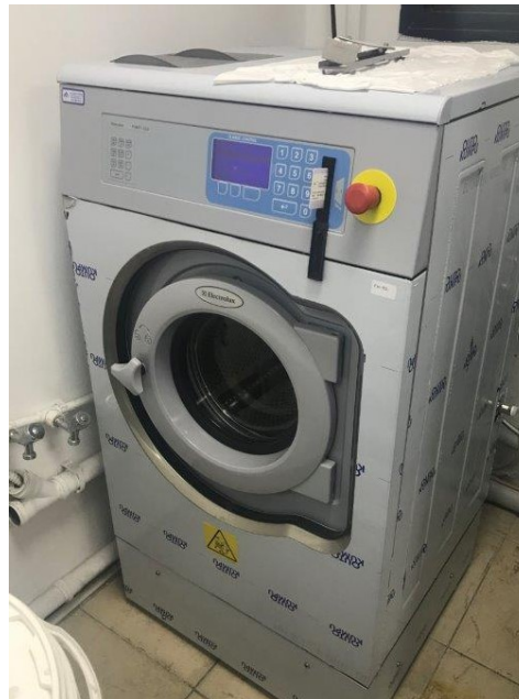
Figure 4.9 James Heal Wascator FOM71CLS test device
