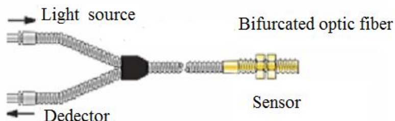
Figure 2.7 Schematic structure of a bifurcated optical fiber.
