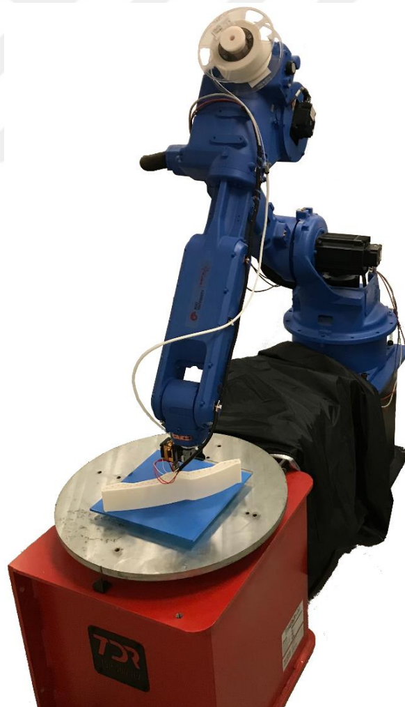
Figure 32. Robotic additive manufacturing setup using Motoman HP20 industrial robot
