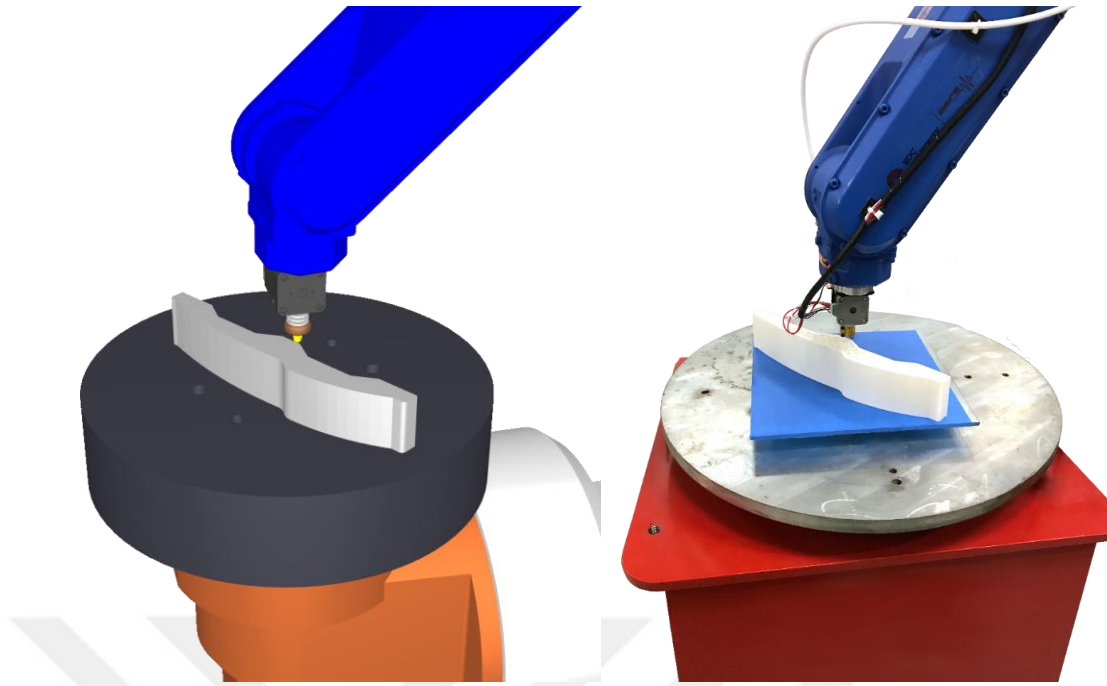
Figure 9. Robotic additive manufacturing setup
