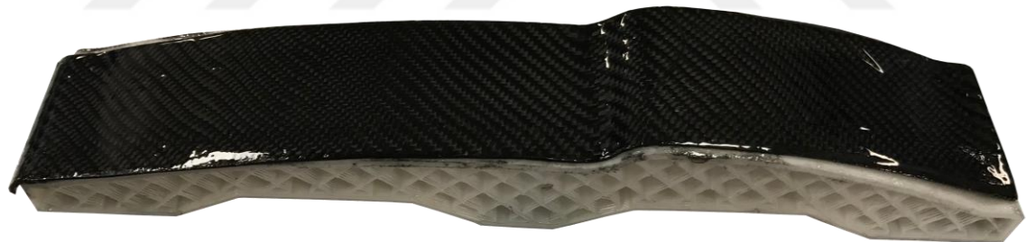
Figure 12. Manufactured carbon fiber part of the Interior panel of an aircraft
