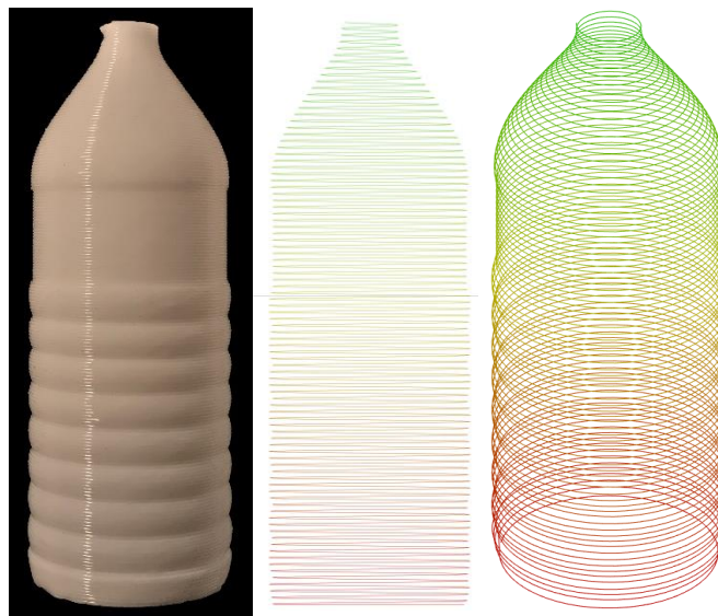
Figure 37. Helical slicing method for a plastic bottle: Fabricated model and the corresponding toolpaths. Dimensions are given as 35 mm width, 35 mm depth, and 90 mm height.
