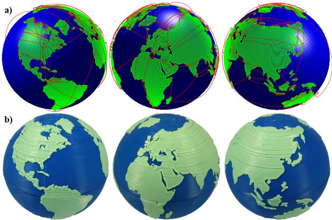
Figure 43. The model of Earth (a) Toolpath for the spherical layer is given in three different angles. The spherical layers are shown with green, the rapid movements are given in red, and the planar base is given in blue. (b) The fabricated model where the planar base is manufactured in two halves with blue filament on top of a bed matching the exact diameter of the base. The spherical layer is on the planar base using the green filament.
