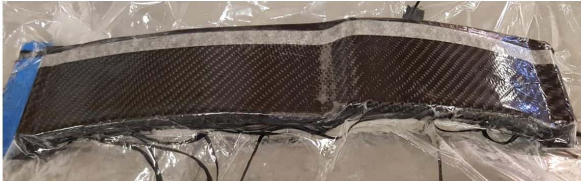
Figure 11. Laid-up part curing inside the vacuum bag
