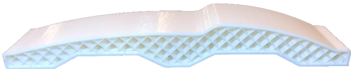
Figure 10. AM tooling for the Interior panel of an aircraft
