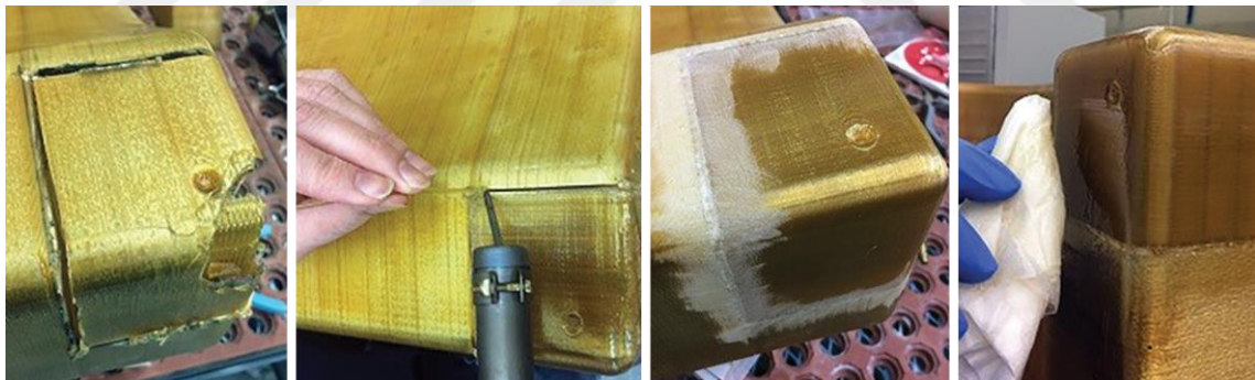
Figure 6. AM Tool repairing process [23]
