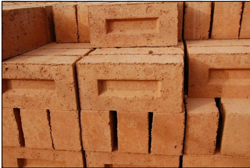
Figure 3.2: Compressed Stabilized Laterite Brick Sample (Arad Branding 2024).
