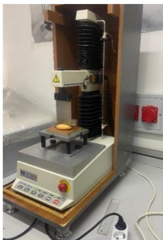
Figure 3.8. Biscuit Measurement with TA-XT Plus Device .
