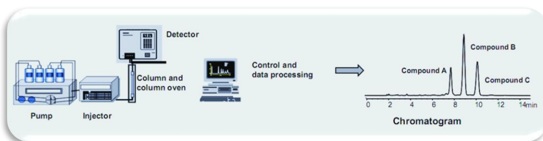
Figure 1.14. Flow scheme for HPLC (Anonymous 4, 2013)
