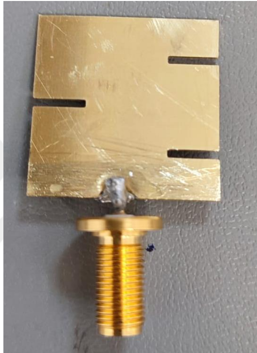
Figure 5. 2 Radiating element is connected to SMA connector
