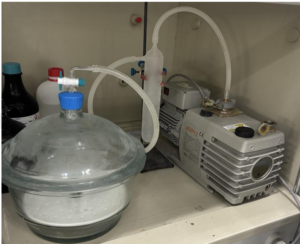
Figure 14: The setup for lyophilization. The desiccator (left) and vacuum pump (right) are seen in the figure, and there are linkages between them.
