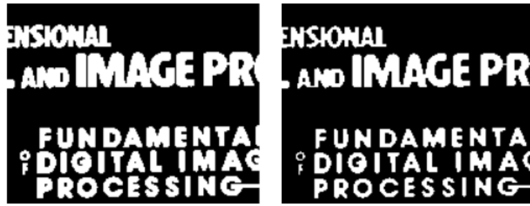
Figure 23: Left image is binary image and the right image is the result after erosion with 2*2 structuring element
