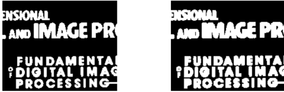
Figure 21: Left image is binary image and the right image is the result after dilation with 2*2 structuring element
