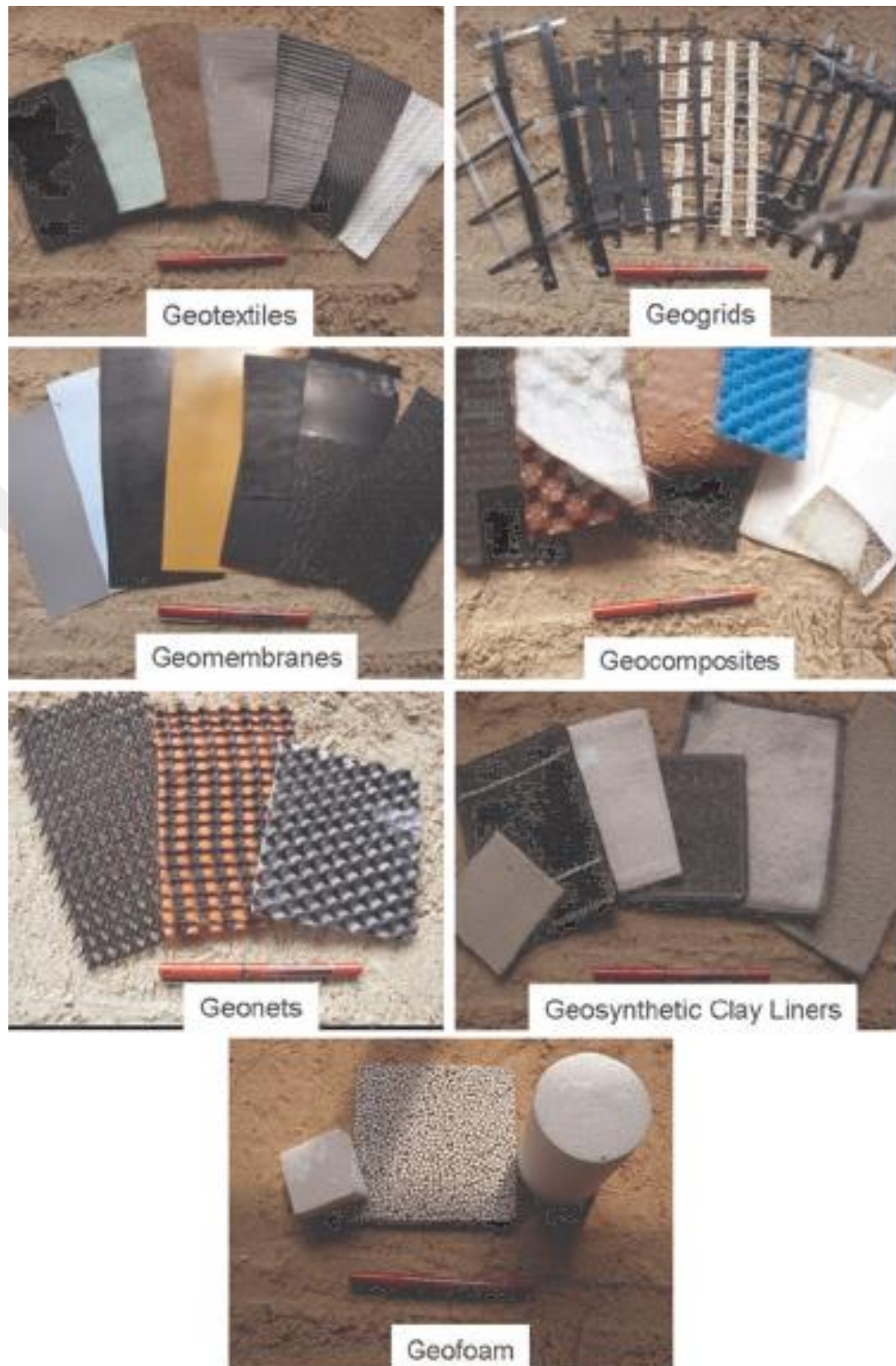
Figure 3.3. Typical geosynthetic materials types [30].
