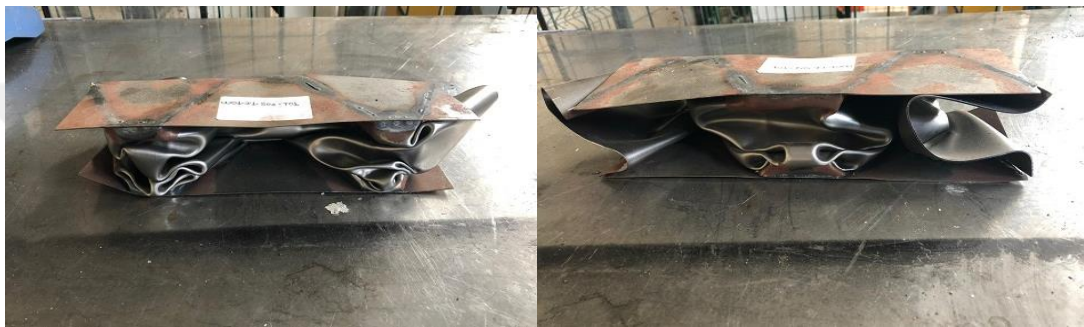
Figure 4.9. W01-I1.0-S03-T01 sample after deformation Front & Back side view
