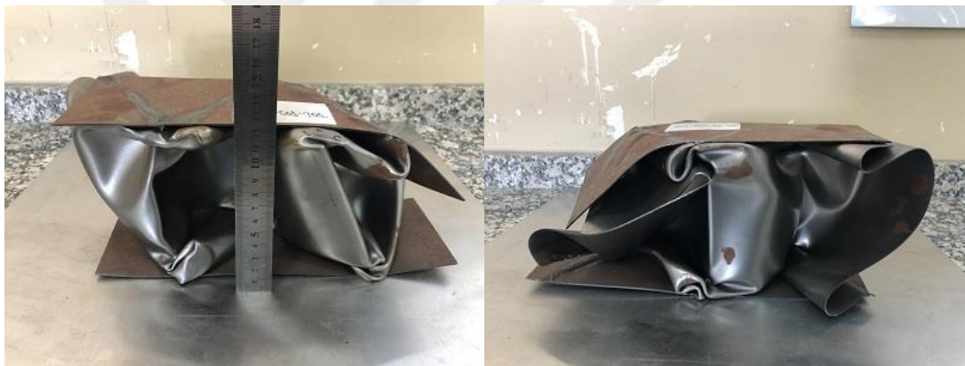
Figure 4.16. W02-I1.0-S01-T01 sample's front and back view after collision
