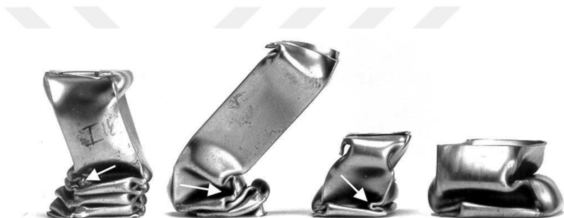
Figure 1.6. Square columns resulting from the development of symmetric and 'inverted' folding modes indicated by white arrows
