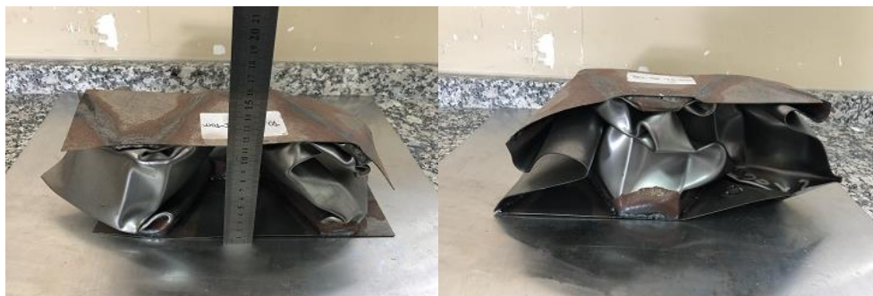
Figure 4.8. W01-I1.0-S02-T01 sample after deformation Front & Back side view
