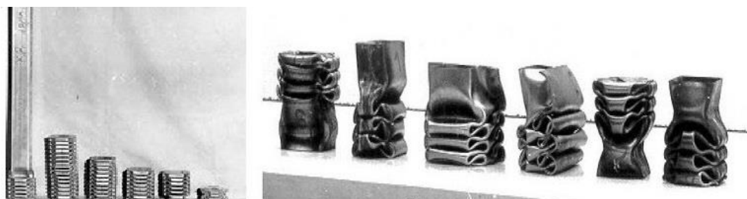
Figure 1.5. Folding of properly triggered elements, often subjected to axial impact loading
