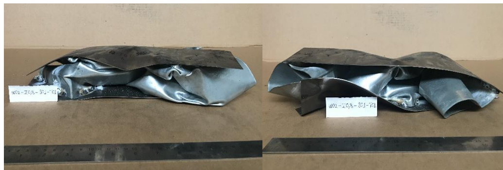
Figure 4.19. W02-I0.8-S01-T01 sample's front and back view after collision
