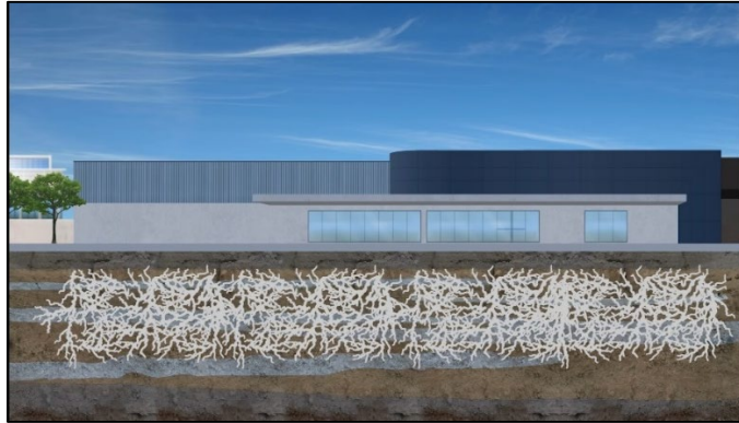
Figure 1.6: Injected Resin Beneath The Structure, 09/2017 New Zealand.
