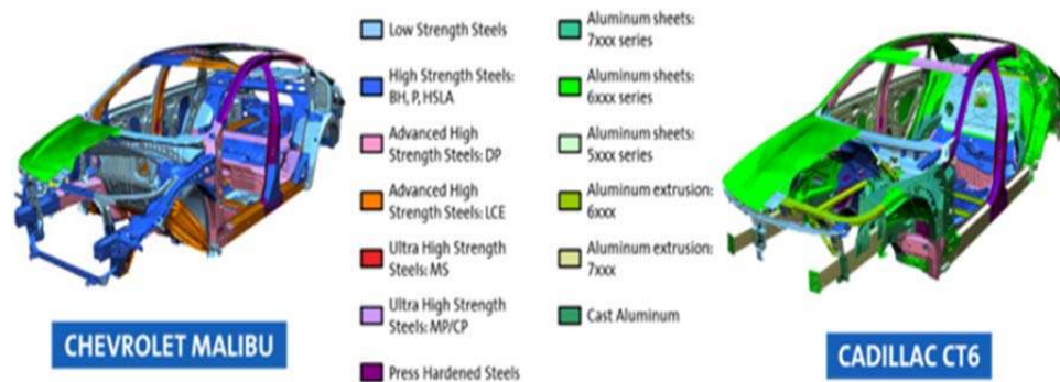
Figure 1.3. Mixed materials BIW (Body in White) for Chevrolet Malibu and Cadillac CT6 (courtesy of General Motors) (Liu et al., 2018)
