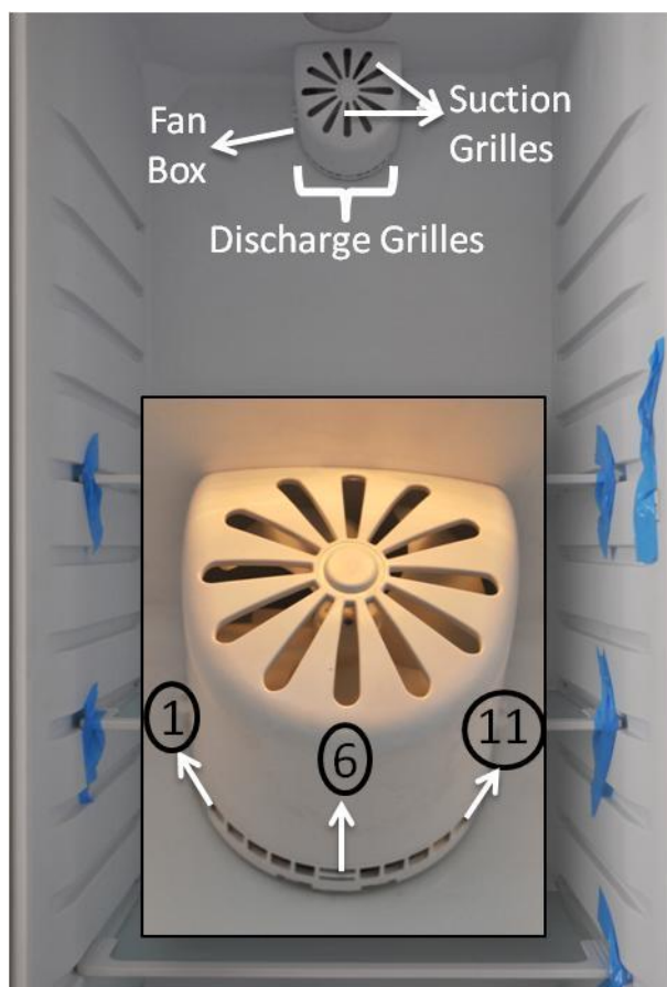
Figure 3.9 The fan box and its grilles positions
