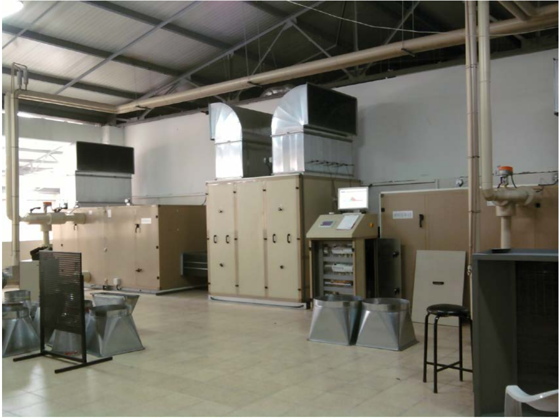
Figure 5.1 Air to air heat exchanger test system
