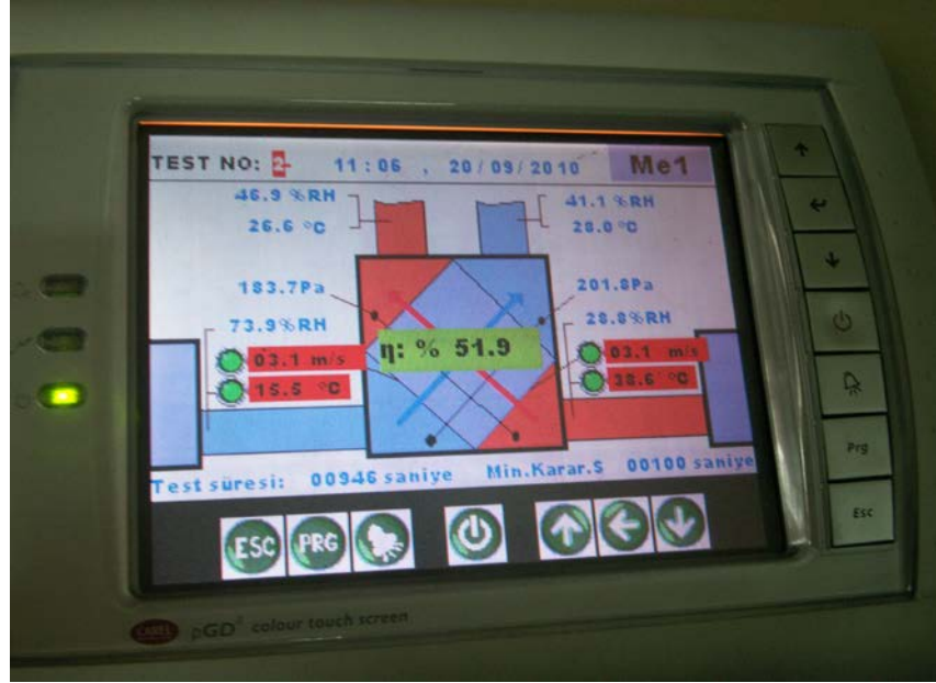
Figure 5.12 Test results that all intended values are supplied
