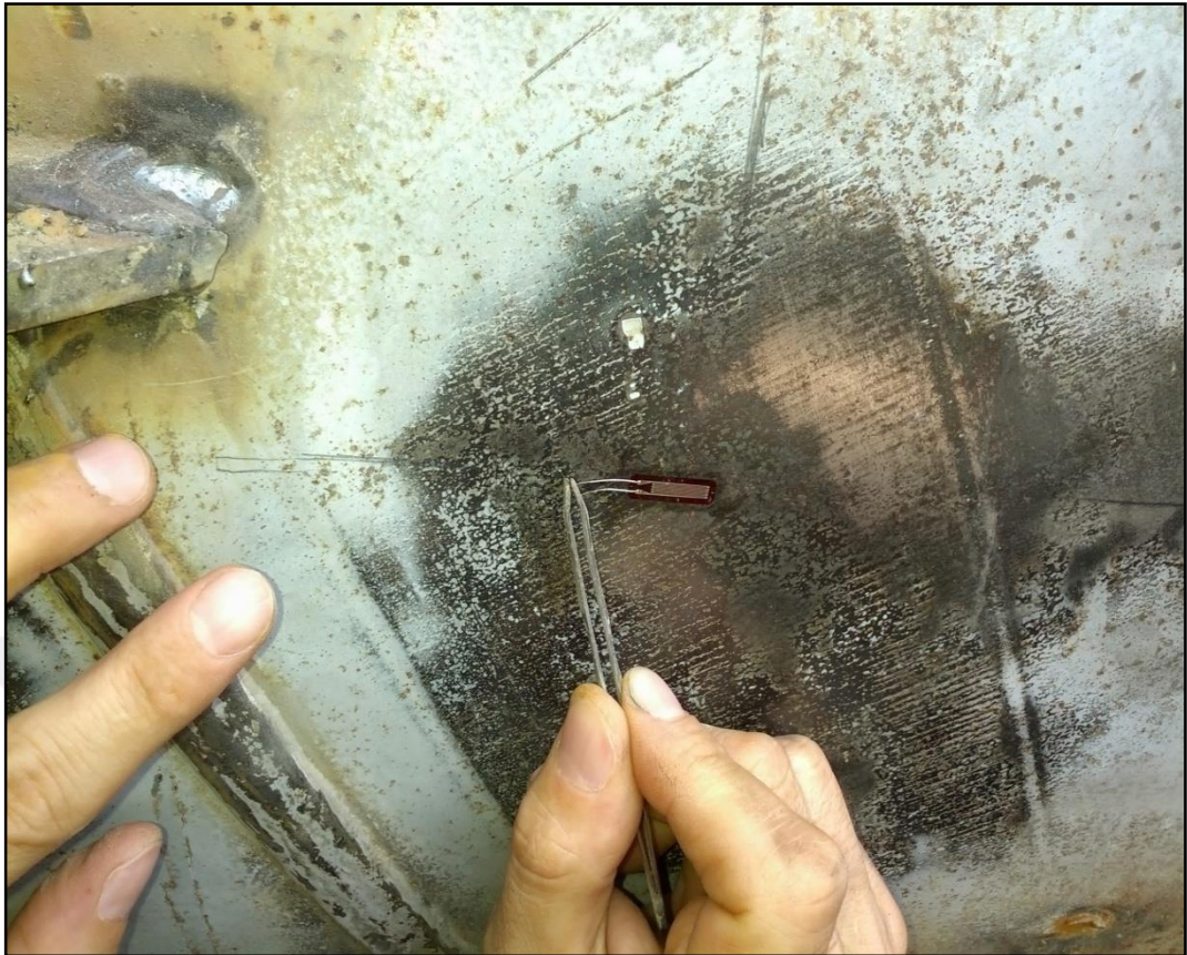
Figure 4.19 Raising the gauge leads
