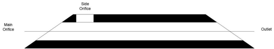
Figure 4.4 Cross-sectional view of ExPress P200 device.
