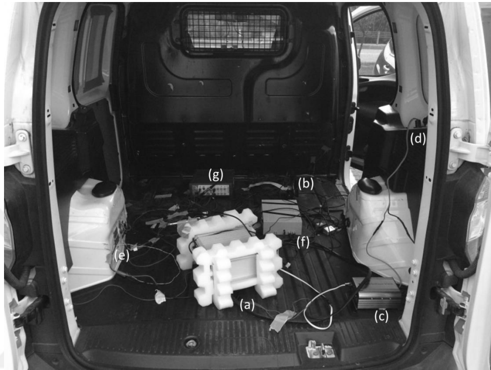
Figure 25 Details of the running vehicle experimental set-up a) Industrial PC b) TFT LCD Screen c) Power Invertor d) DC Outlet Multiplexor e) Piezoelectric Patches f) PZT Amplifier g) Signal Analyzer
