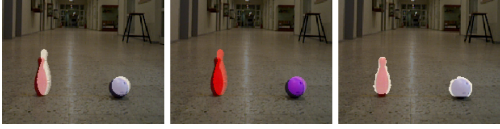
Figure 3.2: Outputs of LINE-MOD (left), LINE-MOD&HS (middle) and Segmentation (right) [24].
