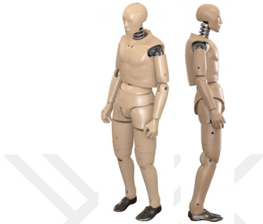
Figure 2.15. 50 th Pedestrian Test Dummy [24]
