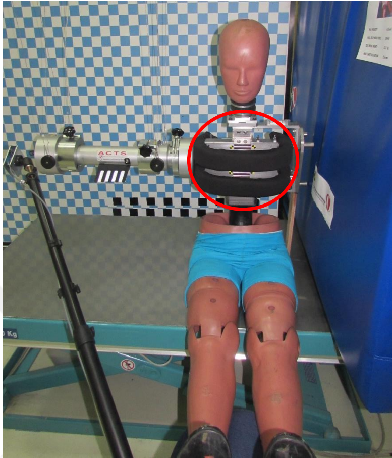
Figure 5.10. ThImp-PED Pendulum Test Set-Up
