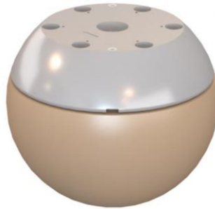
Figure 2.19. Pedestrian Headform Impactor [24]
