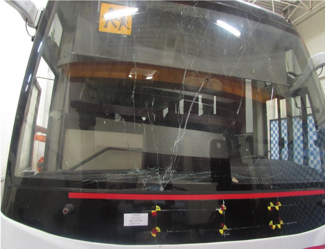
Figure 6.30. Post Test Photograph for Pedestrian Test-4 Showing the Cracks
