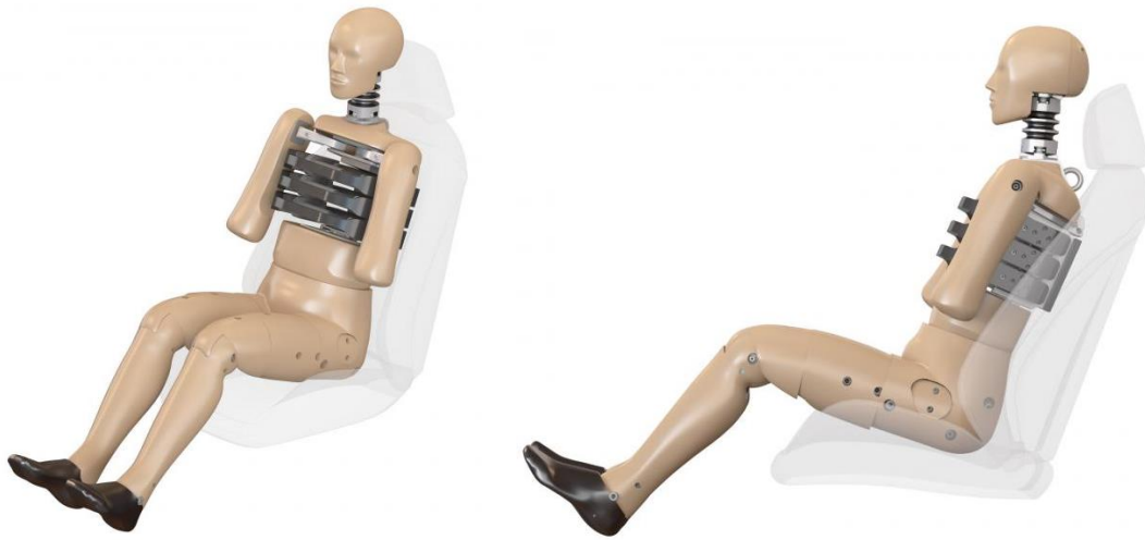
Figure 2.7. ES-2 Crash Test Dummy [24]
