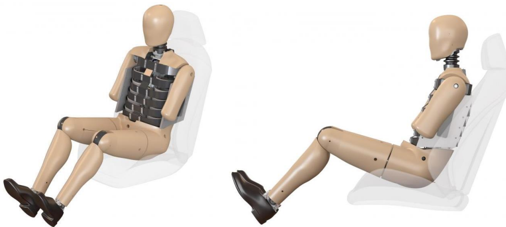
Figure 2.10. WorldSID Crash Test Dummy [24]
