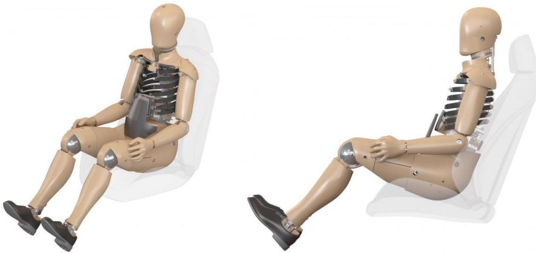
Figure 2.5. THOR 50 th Percentile Male Crash Test Dummy [24]
