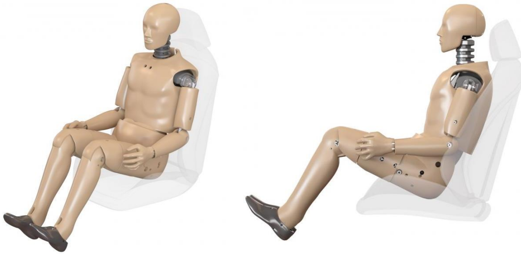
Figure 2.3. Hybrid III 50 th Percentile Male Crash Test Dummy [24]
