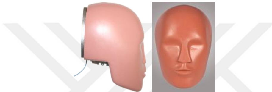
Figure 2.18. Free Motion Headform Used for FMVSS 201U Tests [24]
