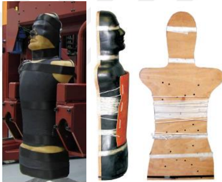
Figure 2.17. Bodyblock Used for ECE R12 Tests [33]
