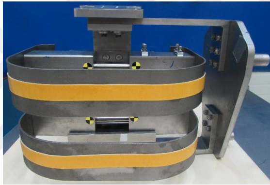
Figure 5.5. Adhesive Tapes for Foam Fixation
