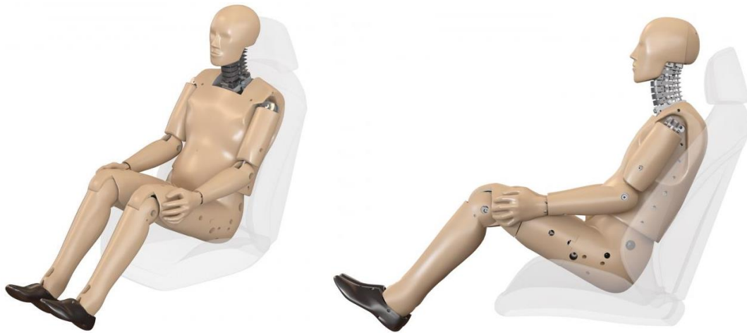
Figure 2.14. BioRID-II Crash Test Dummy [24]
