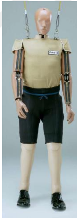
Figure 2.16. POLAR Pedestrian Test Dummy [34]
