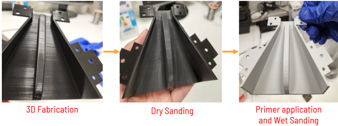
Figure 3.14: Post-Processing of 3D printed pieces.
