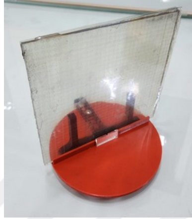
Figure 4.16: Absorber under test, absorber holder (orange) and apparatus (black).
