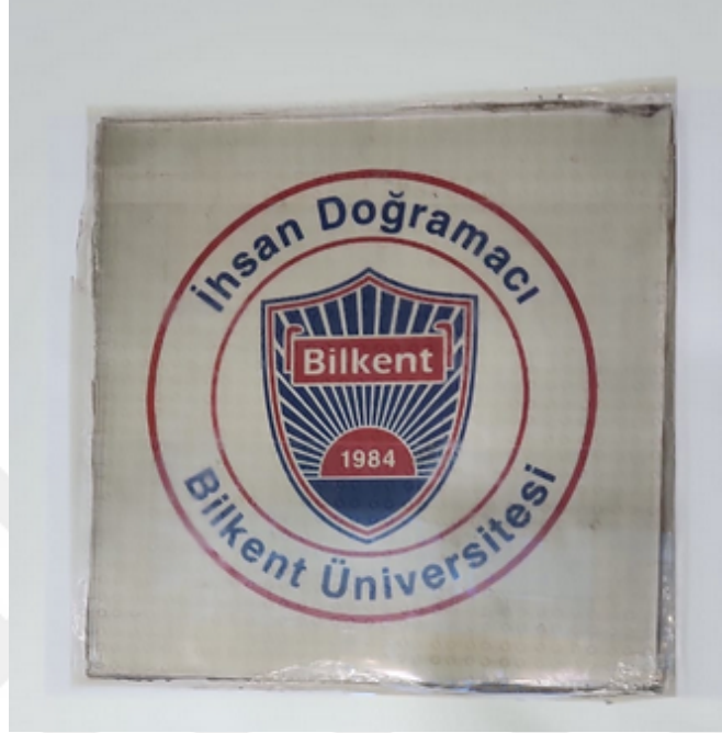
Figure 4.26: Optically transparent absorber placed above Bilkent University logo that can be clearly seen through.
