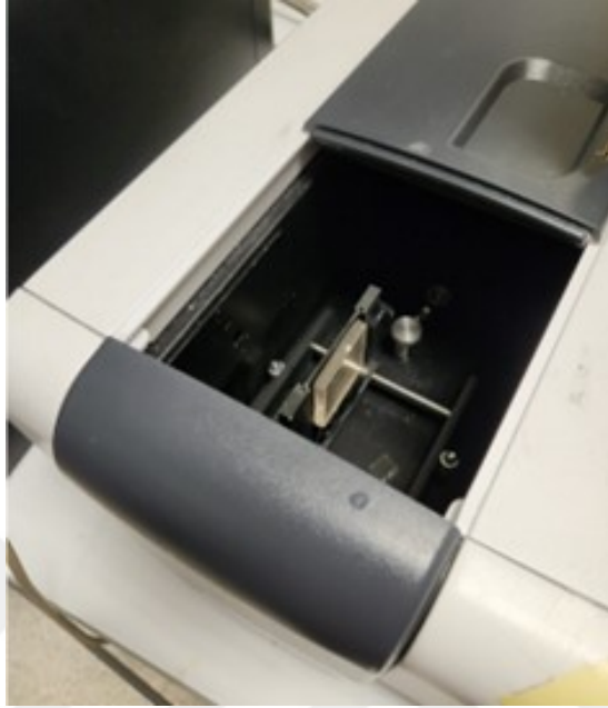
Figure 4.24: Sample placed inside Cary UV-Vis spectrophotometer.
