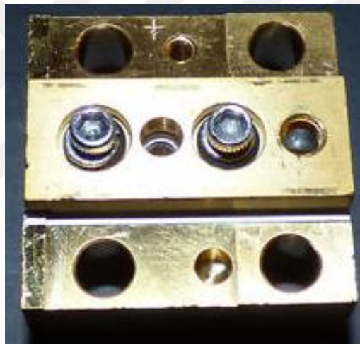
Figure 2.9: Traditional high-power Coherent Laser Diode Bar packages
