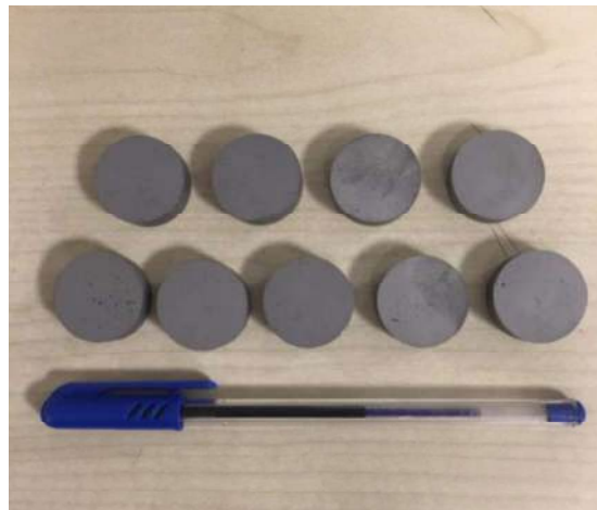
Figure 3.1 Chosen 9 pieces 1.2344 hot work tool steels for study
