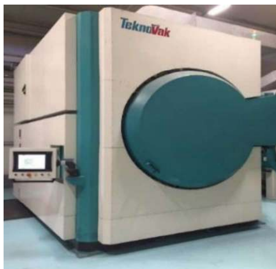
Figure 3.2 Kn controlled gas nitriding furnace
