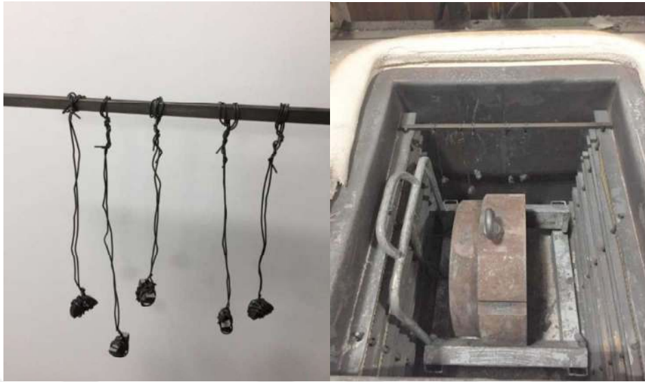
Figure 3.5 Nitrided specimens are suspended in air furnace
