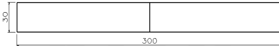
Figure 3.9. Geometry and dimensions of the tensile test specimens used after GMAW
