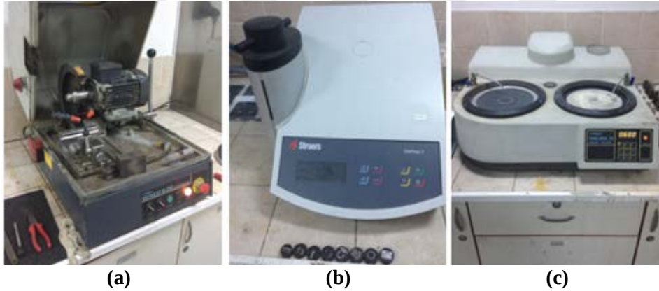
Figure 3.6. The devices which were used to prepare the samples (a) Circular saw, (b) Bakelite forming device and (c) Automated grinding machine
