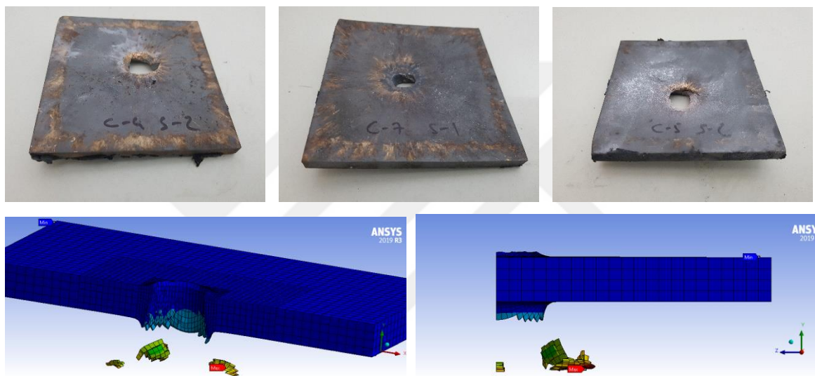
Figure 5.2. Fragmentation in steel coverplate.
