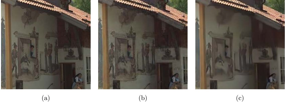
Figure 3.6: Example crop from Kodak dataset: (a) original crop, (b) compressed-decompressed with the proposed network at 0.3347 bpp with 29.89 dB PSNR and 0.9507 SSIM, (c) compressed-decompressed with GDN network at 0.2730 bpp with 30.0169 dB PSNR and 0.9424 SSIM. Although both images are at similar quality levels, Figure (c) is more blurry than Figure (b) on paintings on the wall. Both images are quantized with the unit quantization step.
