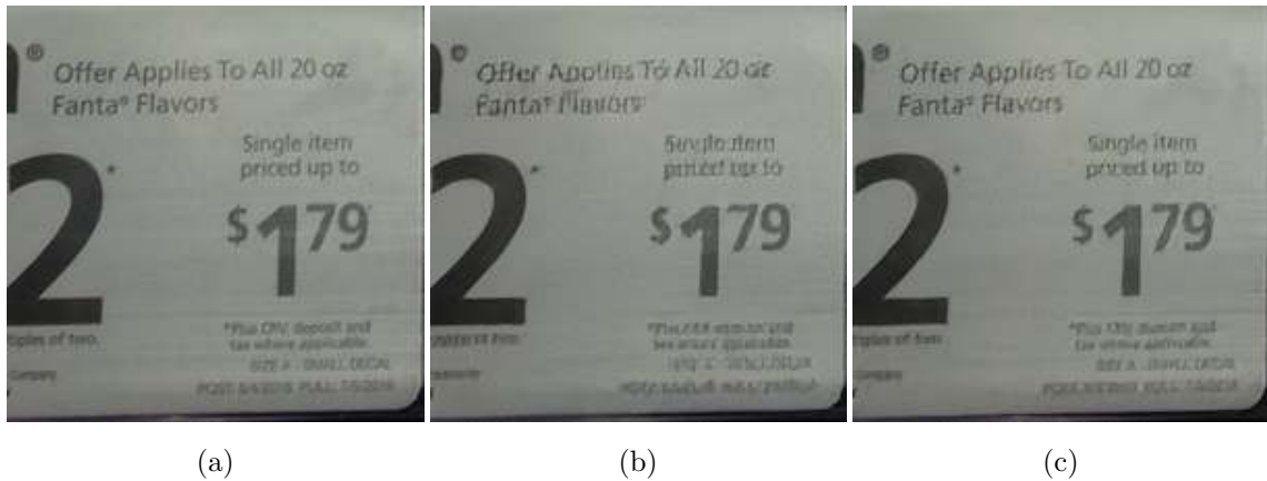
Figure 4.6: Example crop from CLIC 2018 test set: (a) original crop, (b) output of HIFIC-RDP3, (c) output of HIFIC-RDP4. (b) is encoded by HIFIC-lo at 0.1437 bpp, 32 dB PSNR, LPIPS 0.1980. (c) is encoded by HIFIC-mi at 0.2706 bpp, 34.5 dB PSNR, LPIPS 0.1481.
