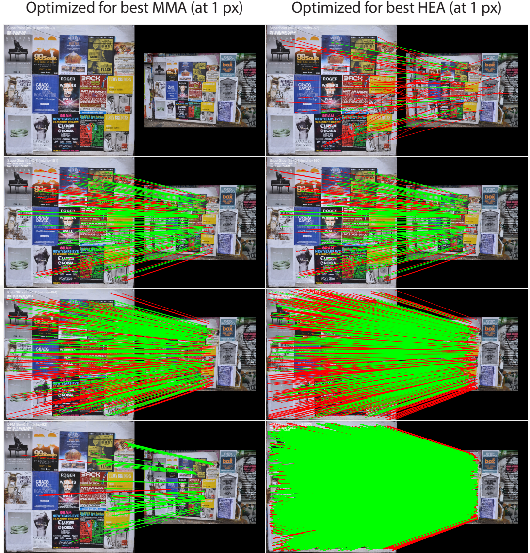
Figure 4.8: Visual Illustration of results of Learning-based Algorithms Super-Point, SuperGlue, Patch2Pix, and DFM optimized for giving the best MMA (the left column) and the best HEA (the right column) under 1-pixel threshold on the image pair posters 1 & 4
