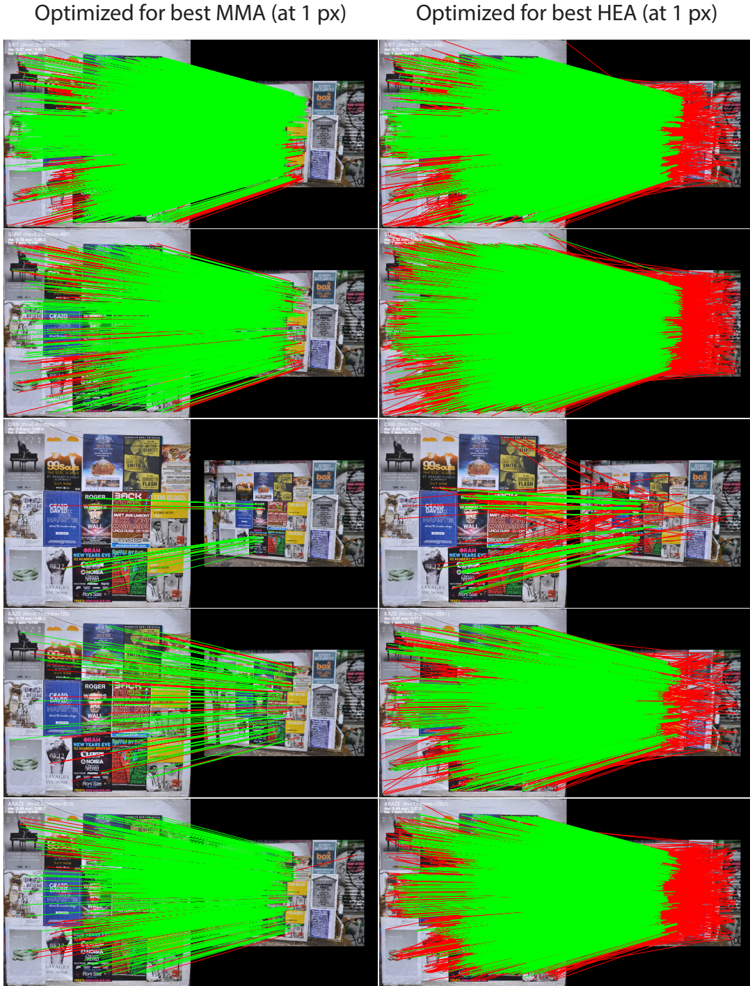
Figure 4.7: Visual Illustration of results of Classical Algorithms SIFT, SURF, ORB, KAZE, and AKAZE optimized for giving the best MMA (the left column) and the best HEA (the right column) under 1-pixel threshold on the image pair posters 1 & 4
