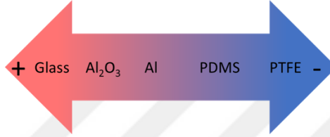
Figure 1. 1. An example of a triboelectric series of materials, adapted from [10] and [11].
