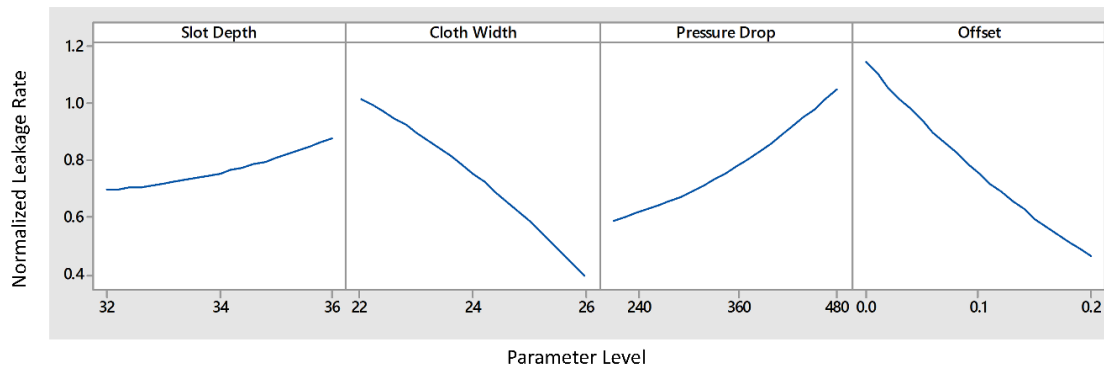
Figure 6.8: The effect plots for normalized leakage rate (Box-Behnken designs with four outliers)
