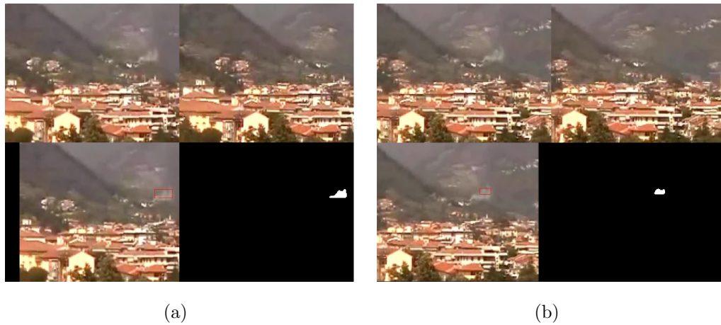
Figure 5.8: Wildfire detection results for two different frame and key-frame pairs using the 360° coverage video sequence. Top-left image is the current frame, top-right image is the corresponding key-frame, bottom-left image is the registered current image, bottom-right image is the candidate smoke region.
