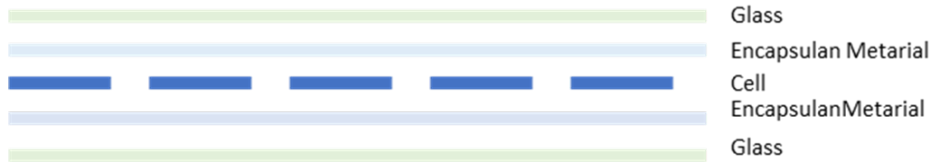
b) Glass Glass Module Structure
