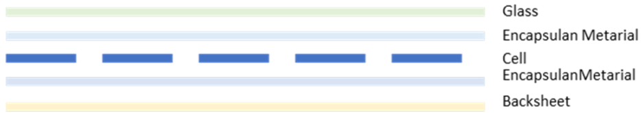
a) Glass Backsheet Module Structure
