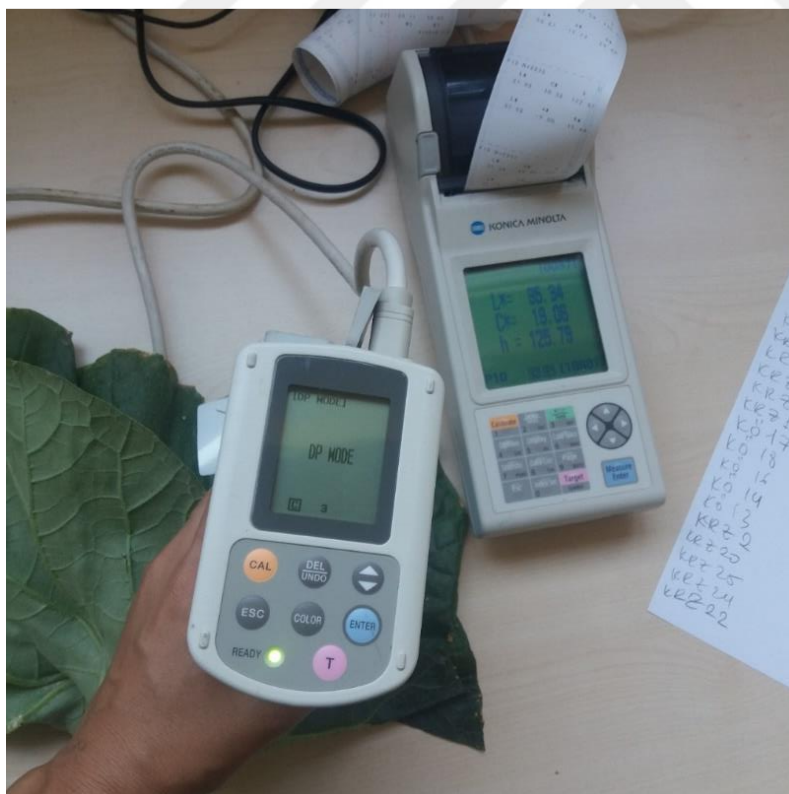
Figure 3.10. Leaf color measurement with portable spectrophotometer
