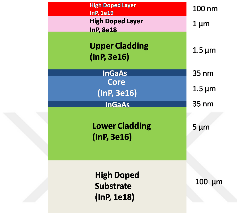
Figure 2.14 Waveguide design illustration of fabricated device
