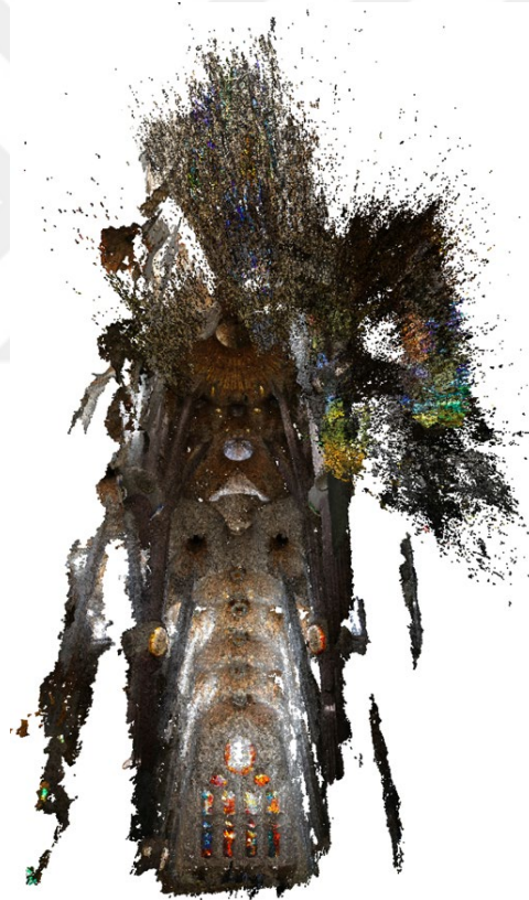
Figure 4.9. Still image showing the central nave of La Sagrada Familia, Barcelona, from the partial dense point cloud model produced in January 2020.
