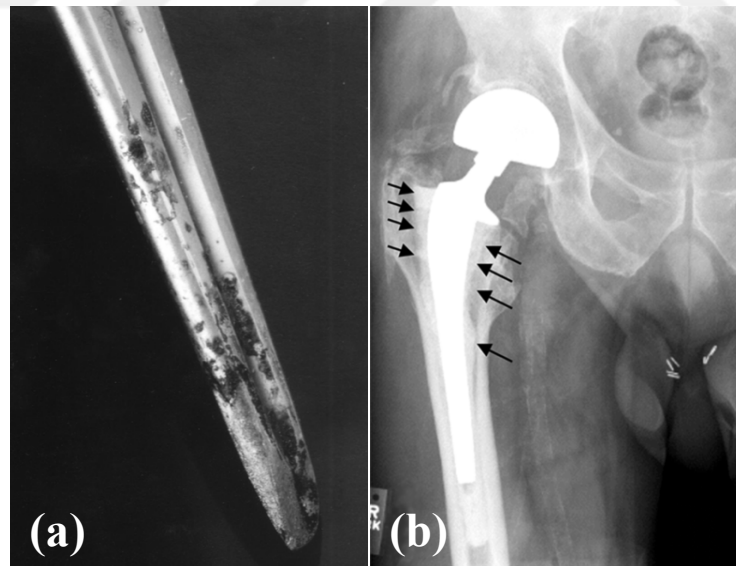
Figure 2.2 a) Corrosion and b) bone loosening in hip implant [18]
