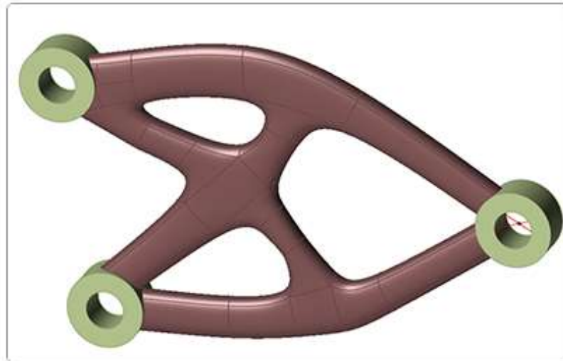
Figure 2.2: Topology Optimized Bracket [5].
