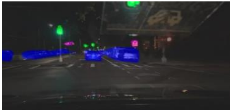
Figure 4.8: Visualization of the traffic object localization result. Green color indicates green light, dark purple indicates traffic signs and blue indicates dynamic objects.
