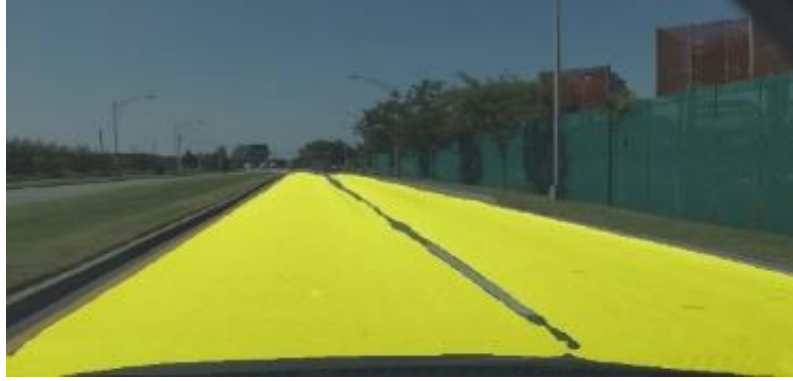
Figure 4.2: Visualization of the drivable area segmentation result. Each lane is separated in terms of drivable area.
