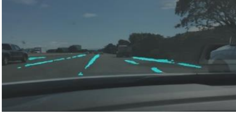
Figure 4.5: Visualization of the lane line detection result. Dashed lines are detected.
