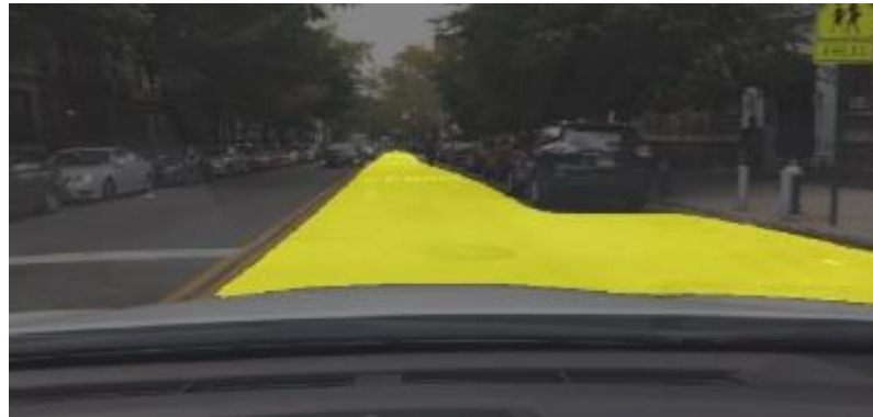
Figure 4.1: Visualization of the drivable area segmentation result. In two-way road case, incoming lane is not segmented.
