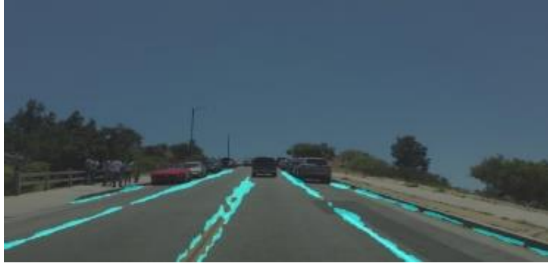
Figure 4.4: Visualization of the lane line detection result. Road curbs and lane lines are detected. These are the direct masks from predictions and are not post processed by any means of line fitting.
