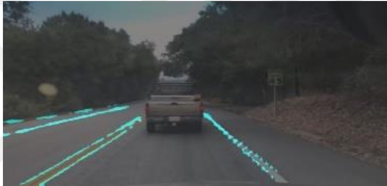
Figure 4.6: Another visualization of the lane line detection result.
