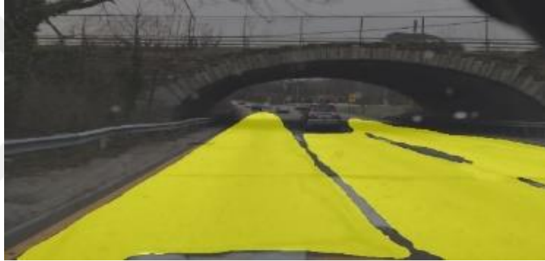
Figure 4.3: Another visualization of the drivable area segmentation results that shows each lane is separated in terms of drivable area.
