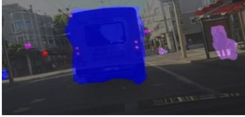
Figure 4.9: Another visualization of the traffic object localization result. Red color indicates red light, dark purple indicates traffic signs, magenta indicates pedestrians and blue indicates dynamic objects.
