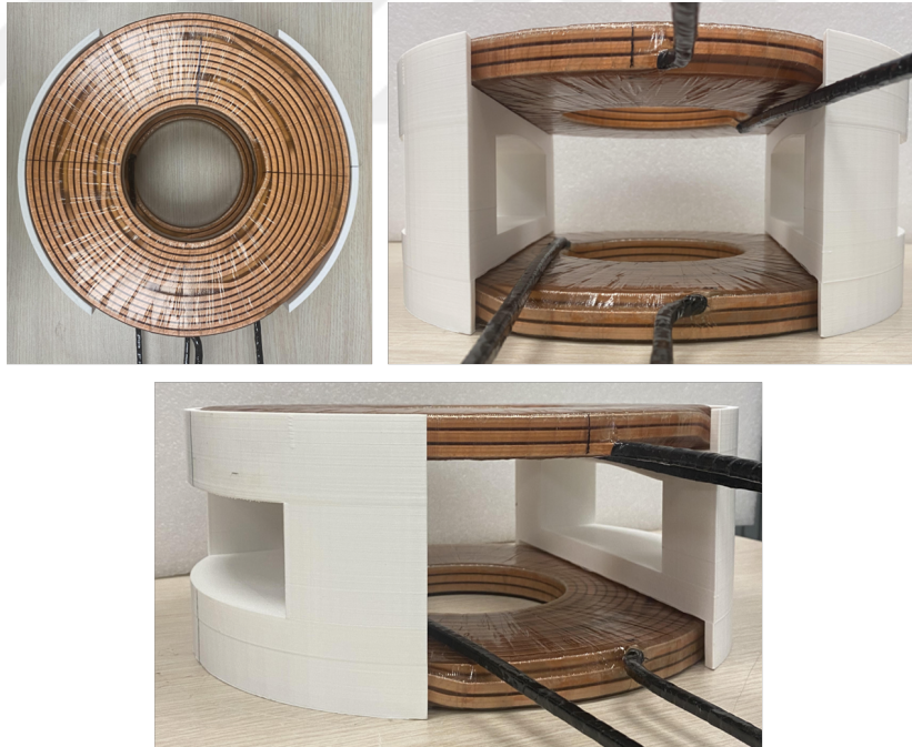
Figure 3.6: C_{z1} coil group. The 3D-printed supports are used to align upper and lower coils.
