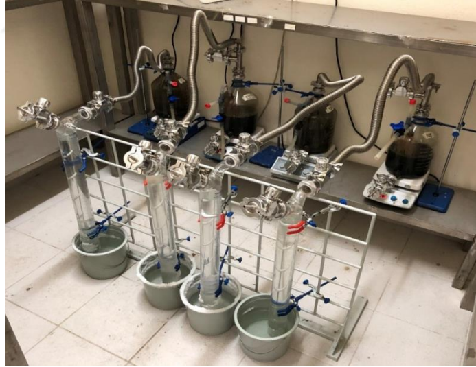
Figure 3.2. Pictures of single-stage anaerobic digesters operated in the study
