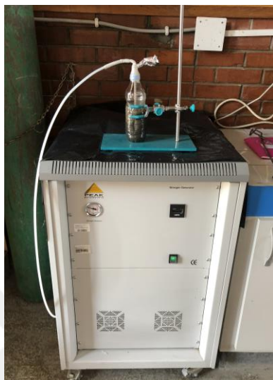
Figure 3.6. Nitrogen generator used in the study
