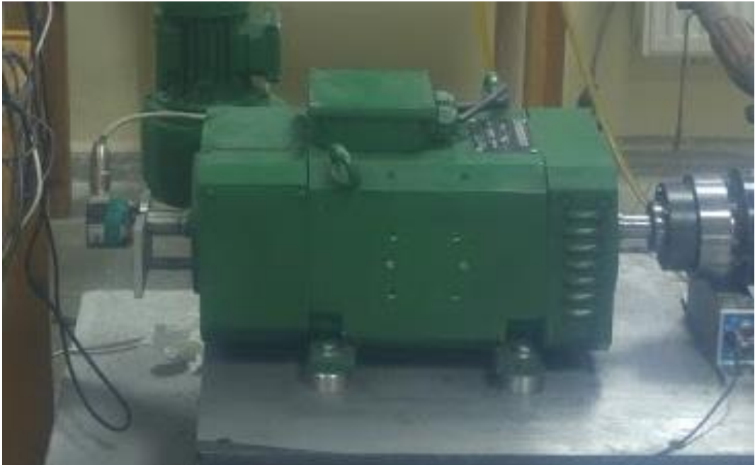
Şekil 5.4. Kemsan marka Direct Current Motor (DC) dinamometre.
