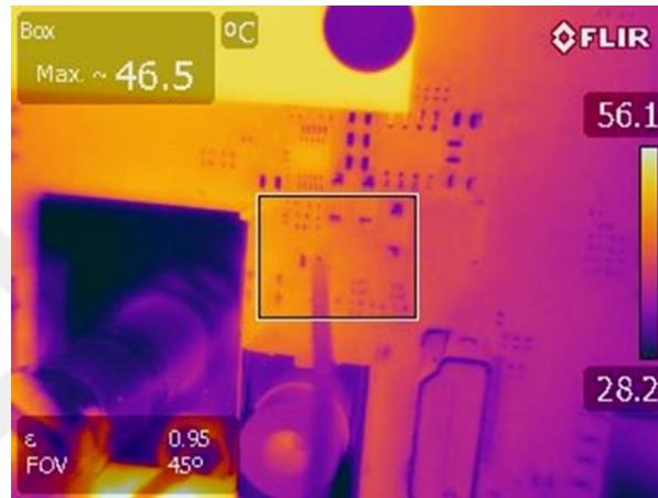
Figure 2.5: Thermal camera image of the LNB Power circuit. The maximum temperature is measured as 46.5°C.
