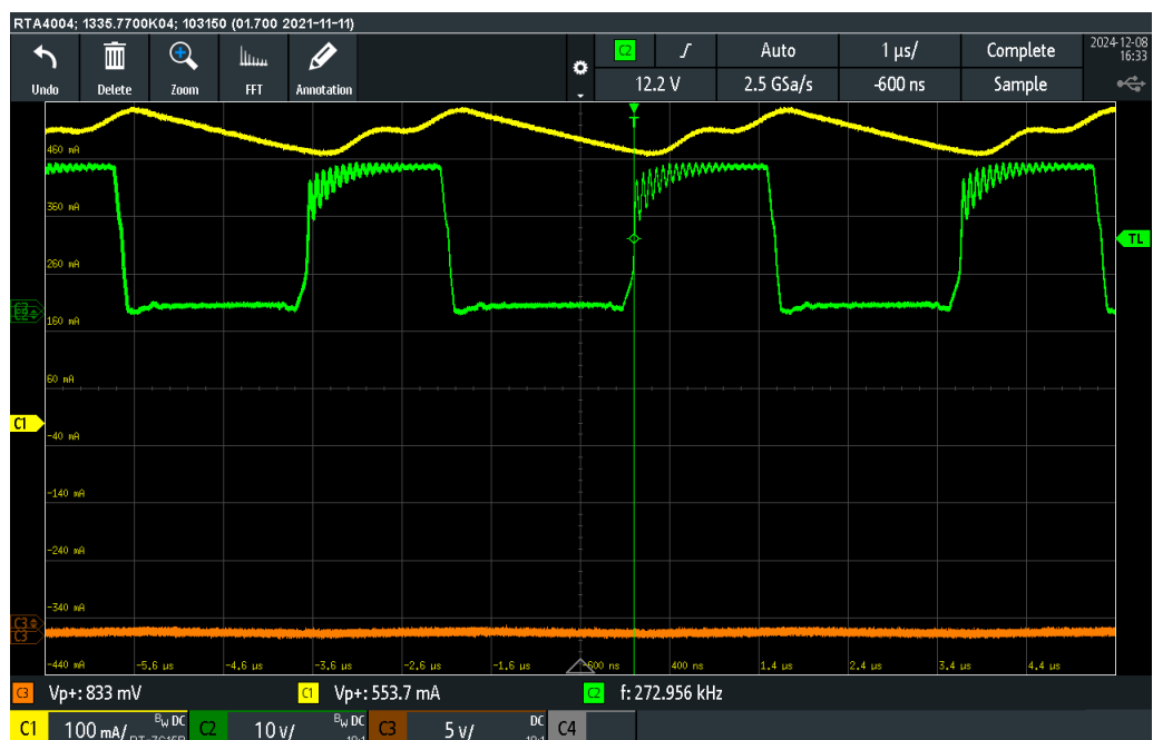
Figure 4.14: Short Circuit Condition
