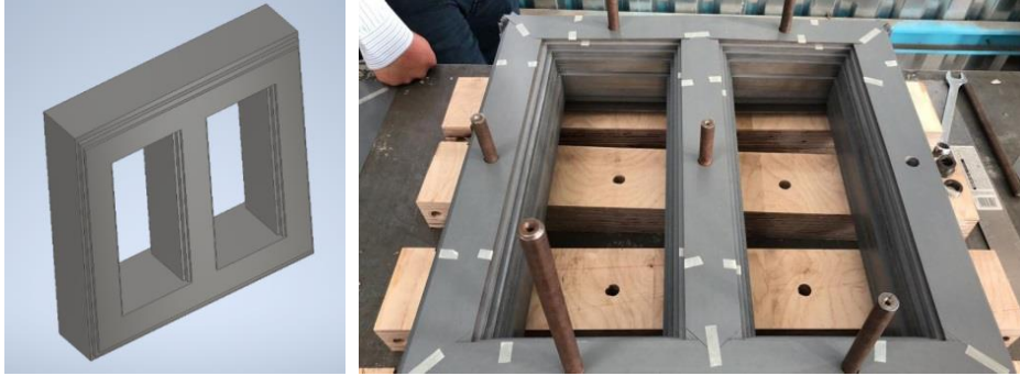
Figure 2.6. Core of a transformer on a 3D design program and in a real production
