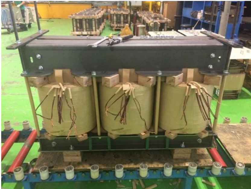
Figure 2.7. Assembly of a coils and core of a transformer.
