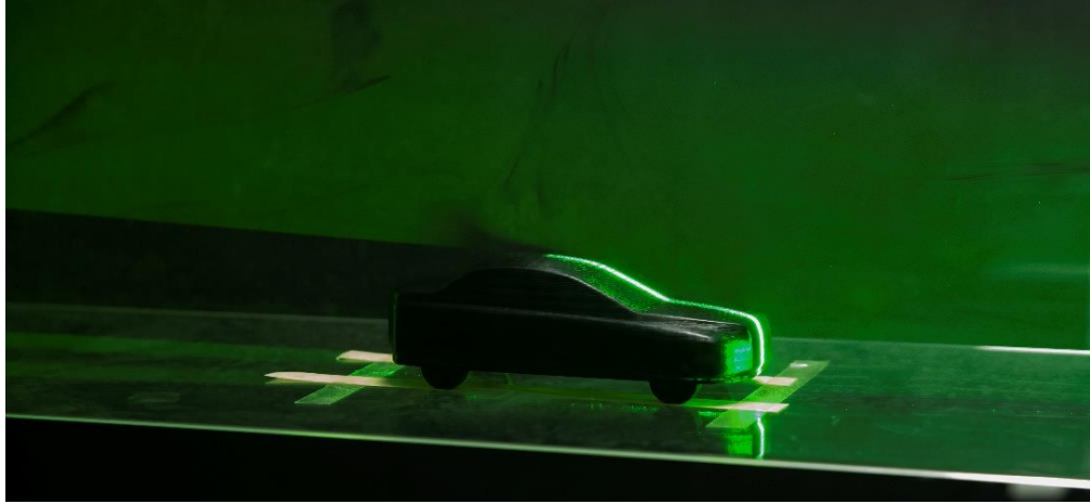
Figure 4.15 Image of Vehicle B captured during the PIV experiments (Personal archive, 2019)
