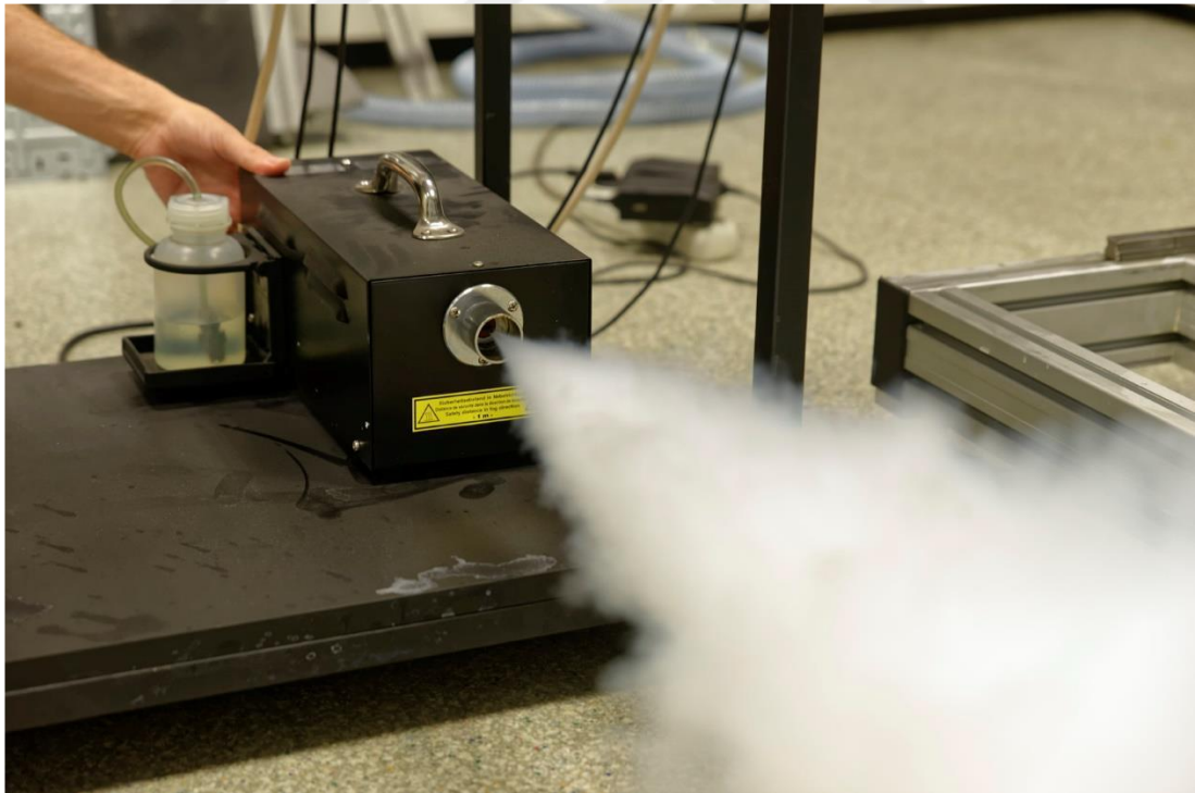
Figure 4.9 Photo of seed generator used in this study (Özer, 2017)
