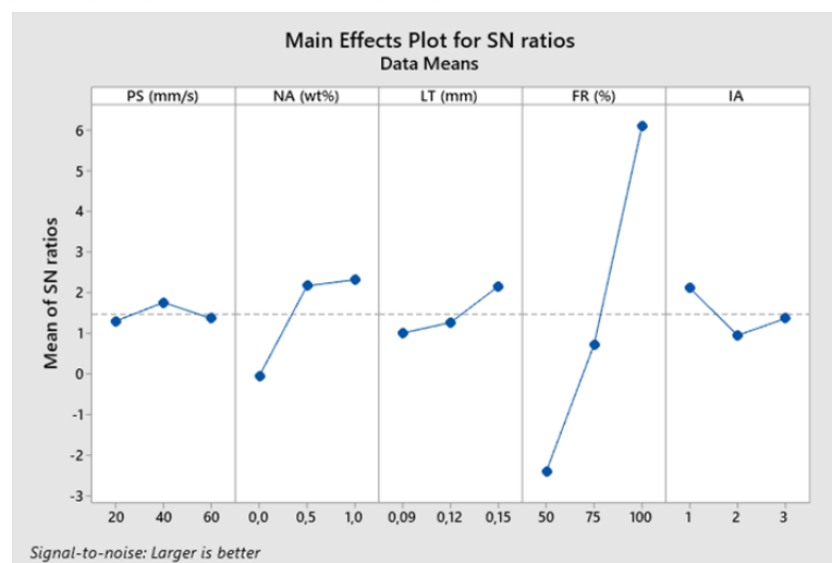
Figure 4.44. Taguchi analysis for total strain energy release rate ( J_T ) in the Mode I/II.
