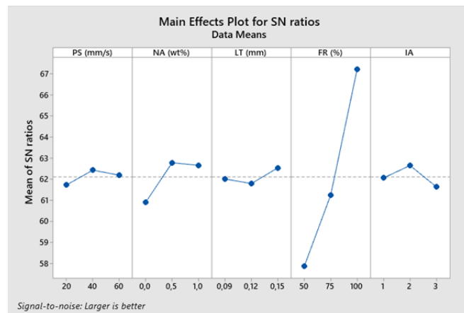
Figure 4.42. Taguchi analysis for critical load ( P_C ) in the Mode I/II
