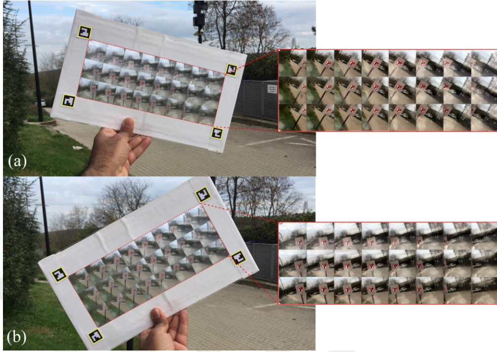
Figure 4.7. The implementation of the surface detection tracking module on two different images. The captured image is processed to detect the corner of the surface and extract the captured perspective views.
