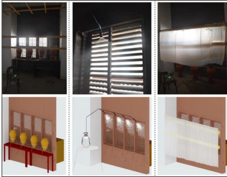
Figure 3.20: Different Model Configurations of Passive Cooling Strategies with the Mashrabiya.
