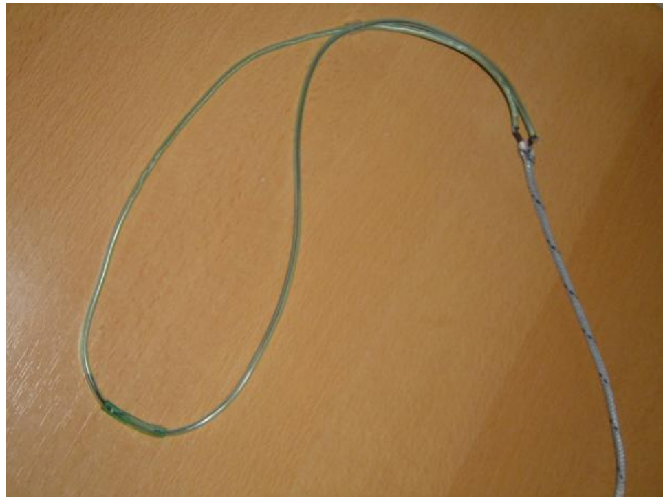
Figure 2.9: Implementation of the Thermocouple Probe
