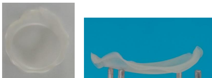
Figure 30. 4 wt % pure PEBAX membrane cast at room conditions in the winter
