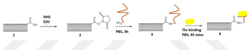
Figure 3.2 Thrombin (Thr) aptamer immobilization onto MWCNTs surface by EDC/NHS crosslinkers and Thr binding to the aptamer
