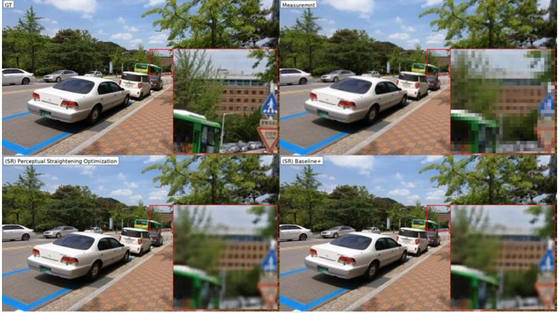
Figure 4.19: comparison of Perceptual Straightening Optimization versus Baseline+ on REDS dataset
