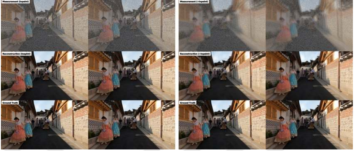
Figure 4.16: Representative comparison of two sequential frames from REDS4 dataset, Left: Inpaint, right: Inpaint+ tasks. From top to bottom: measurement, reconstructed by Baseline (VISION-XL), and ground truth.
